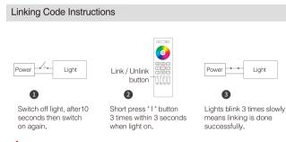
Linking failed if light is not blinking slowly, Please follow above steps again. Linking falled it light to not blinking 6.5..., (Note: Light that have linked can't link again)
