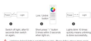
Unlinking failed if light is not blinking quickly, Please follow above steps again. Unlinking railed it light is not billion, a quality, (Note: Light haven't linked that don't need to unlink)
