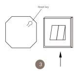
After the wiring of the smart switch is done, long press the "SET" button for 5 seconds or switch ON-OFF the traditional switch 5 times until the indicating light ON.
